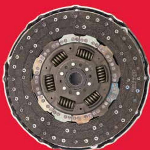
362 mm Diameter Organic Clutch
