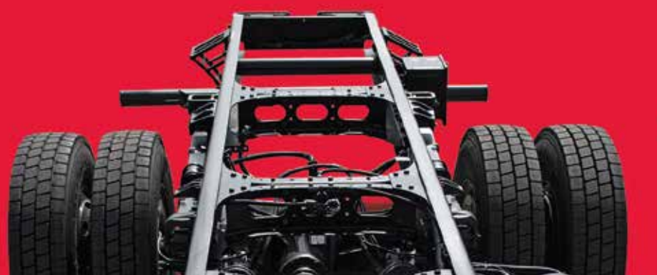
High Strength Low Alloy Material (HSLA 550)
