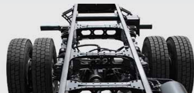
High Strength Low Alloy Material (HSLA 550)
