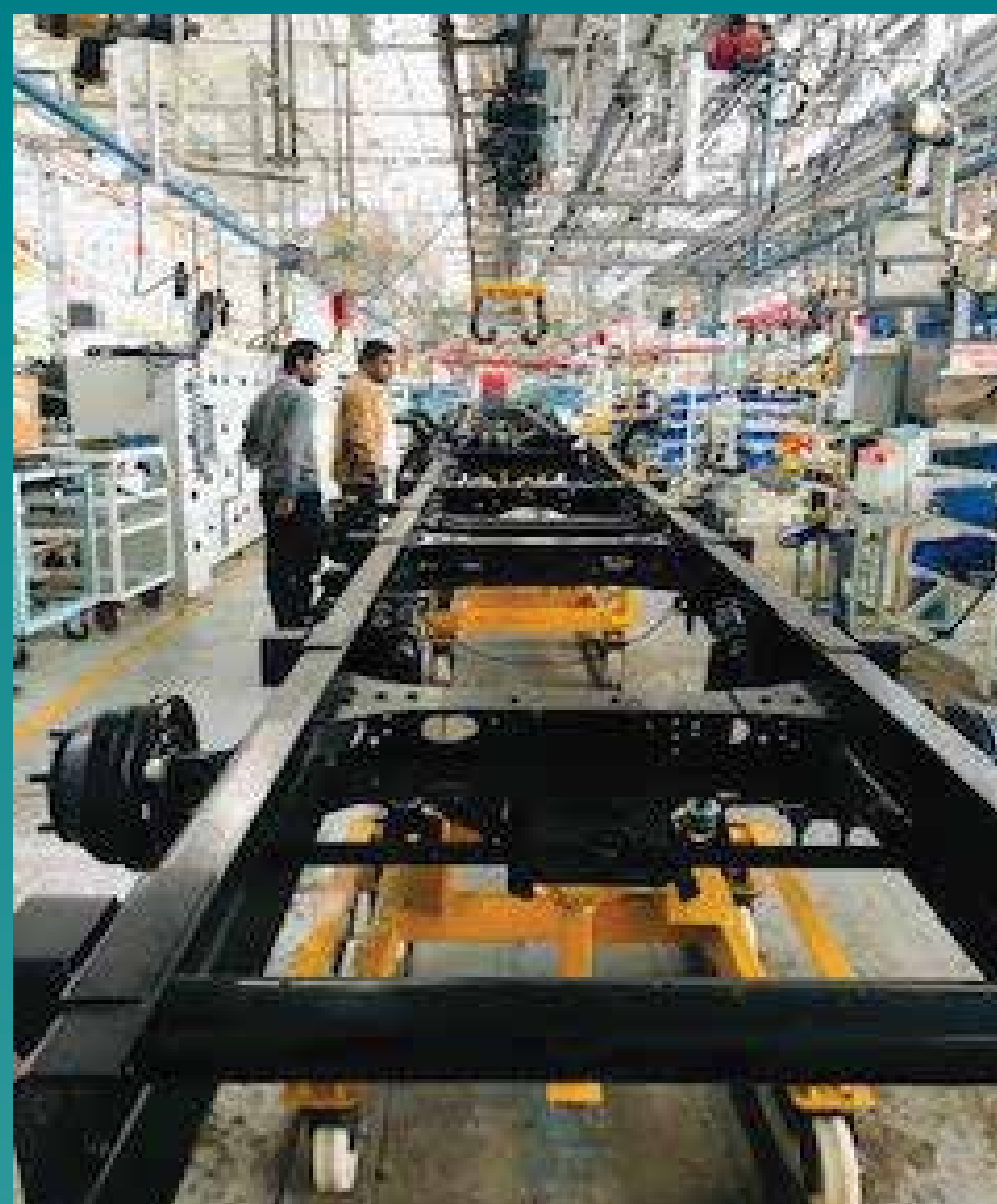
Chassis Frame (High Strength Material 420)
