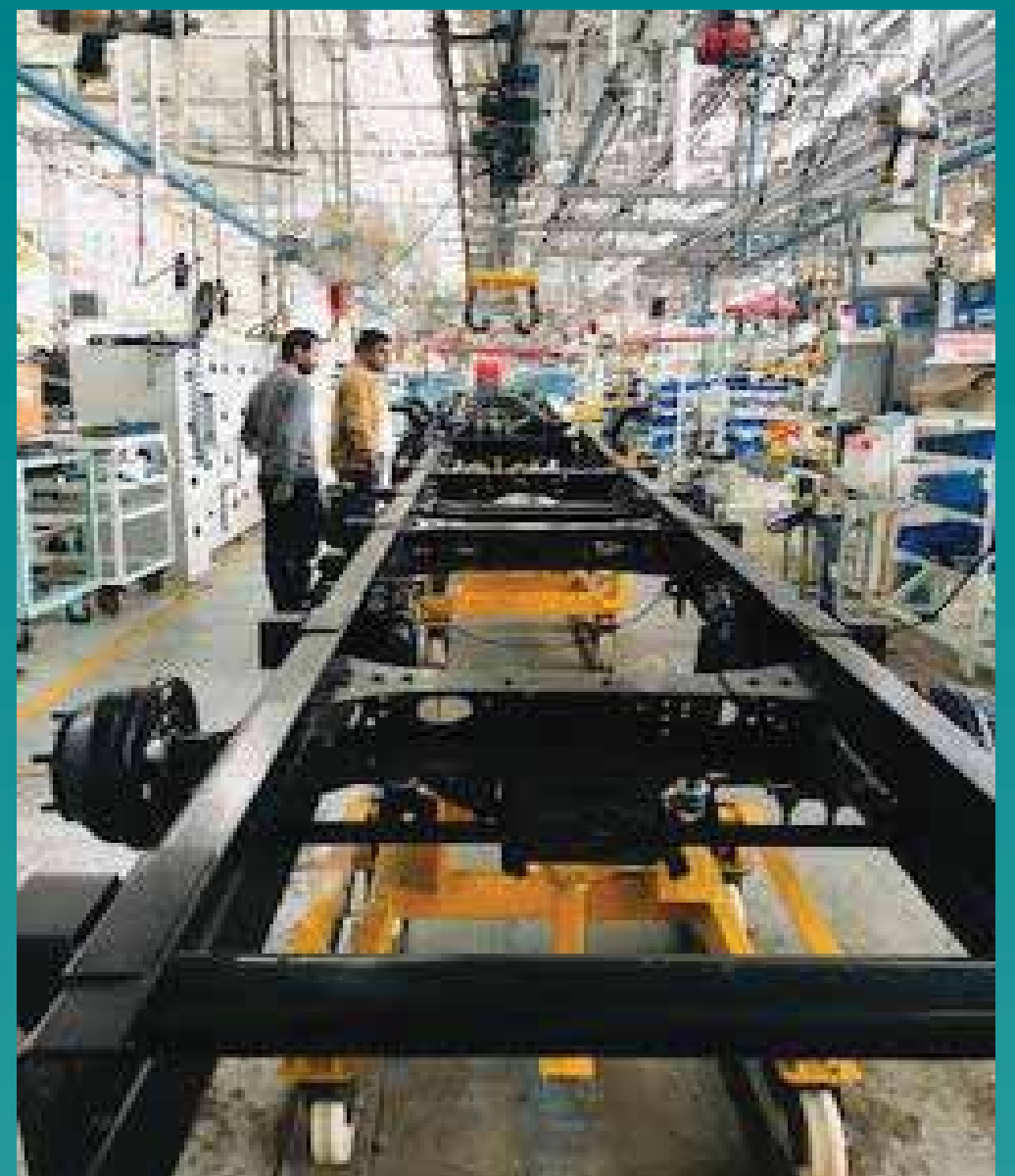
Chassis Frame (High Strength Material 420)
