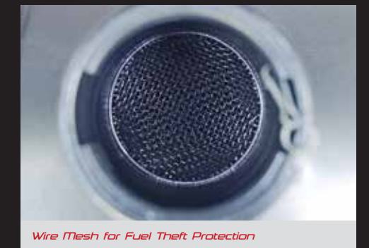
Wire Mesh for Fuel Theft Protection
