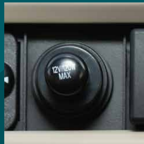
Mobile charging point
